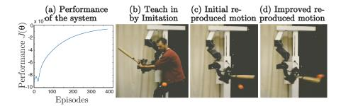
Fig. 2: This figure shows (a) the performance of a baseball swing task when using the motor primitives for learning. In (b), the learning system is initialized by imitation learning, in (c) it is initially failing at reproducing the motor behavior, and (d) after several hundred episodes exhibiting a nicely learned batting.
